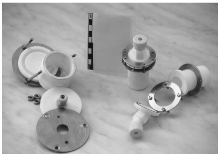
Figure 16 Gas-collector cells prototype 1 (right) and 2 (left); material: porous PTFE with a porosity of 5 and 10 \mu\text{m} and a side thickness of the 3 and 6 mm
