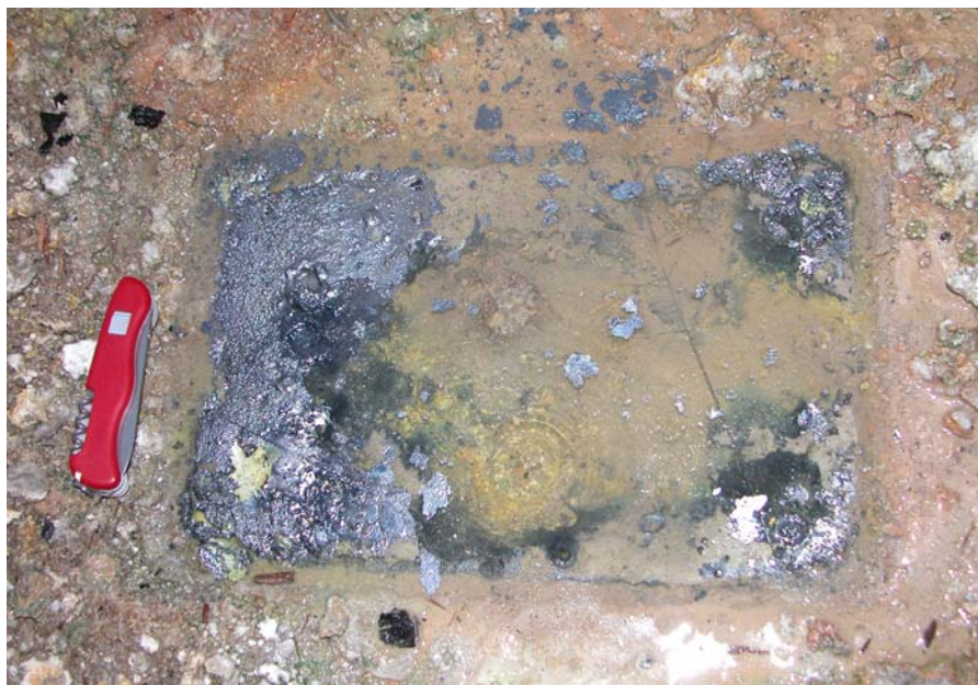
Figure 73 Precipitation of amorphous Fe, S, and As rich material at YNPRH15 underneath a gas hood (33 x 24 x 8 cm) installed for 3 days to sample volatile metallics on SPME
